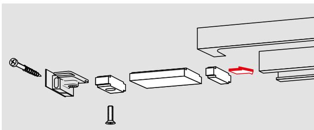
Cushioned limit stay simply slides into the slide channel. Adjustable between 80° and max. 120°. Also suitable for retrofitting.
