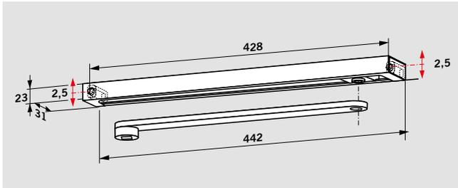
The **G-N** slide channel assembly comprises the main arm, slide channel, slide block, fixings, screws and end caps. The G-N slide channel is non-handed and can be combined with both door closers.
