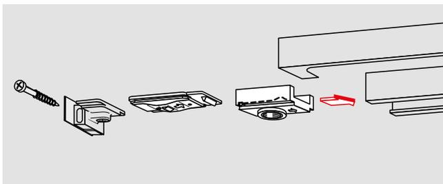
The **RF** mechanical hold-open unit ensures that doors are held open at precisely the correct angle – up to approx. 150° – without any fallback. The hold-open unit can be switched on and off by the user as required, and the pull-off force can be adjusted to suit
