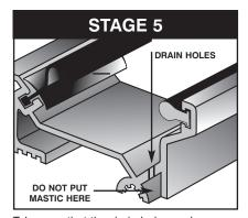
Take care that the drain holes and space behind protector bar are **not** filled with sealant.
