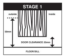
Ensure the door/floor clearance is 25mm. Close door tightly to latch.
