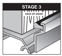
With threshold in position (not fastened at this stage) and the door closed, ensure that the front inside seal is in alignment with the door all along its length. Mark this position on the sill. Drill holes in sill/floor and plug where necessary.
