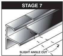
For double doors fit threshold to full width. Cut rain deflector section into two at slight angle as shown.
