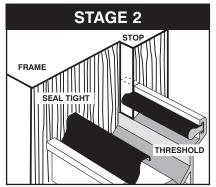
Cut seals and threshold to fit tightly and neatly between frame.
